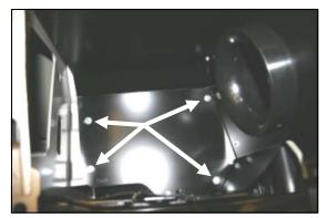
**10.** Install the Airaid **CAD** into the vehicle replacing the factory airbox. Secure the **CAD** using four M6 x 1.25 Hex Bolt (#15), and 1/4" flat washers (#14). Do not over tighten the four bolts.
