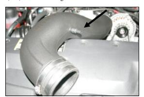
**13.** Install the 1/4" NPT x 3/8" Barb Fitting (#17) into the Airaid Intake Tube as shown. Next install the urethane coupler (#7) onto the throttle body end of the tube using two #64 hose clamps (#16). Tighten *only* the clamp on the tube.
