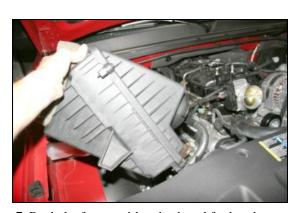
**7.** Rock the factory airbox back and forth to loosen it from the mounting grommets, and remove it from the vehicle.
