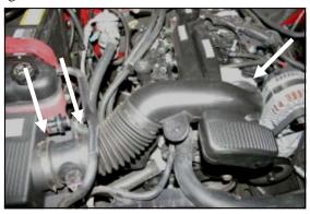
**4.** Loosen three hose clamps. One at each end of the factory intake tube, and one on the Mass Air Flow sensor (MAF) where it clamps to the factory airbox.
