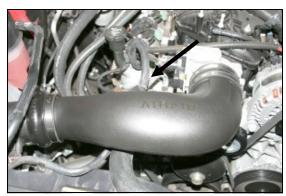
**14.** Install the Airaid Intake Tube into the hump hose first, and then onto the throttle body. Adjust it for fit, and tighten the hose clamps. Next install the 3/8" x 14" breather hose (#8) between the 1/4" NPT x 3/8" barbed fitting in the tube, and the factory port on the valve cover.
